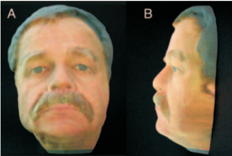
Fig. 3: Colored 3D portrait model of a male subject made by 3D printing; A= front view, B = side view
