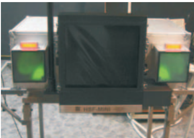
Fig. 2: Holographic camera from the viewpoint of the patient. Left and right are the two illumination ports with the diffuser plates for eyes-safe recording. Centrally located is the mechanical shutter system that covers the holographic plate.
