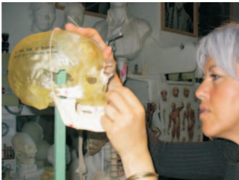
Fig. 6: Stereolithography replica of a skull finding from the Museum for Hamburg History. (©Philippe PLAAILLY/Atelier DAYNES/EURELIOS)
