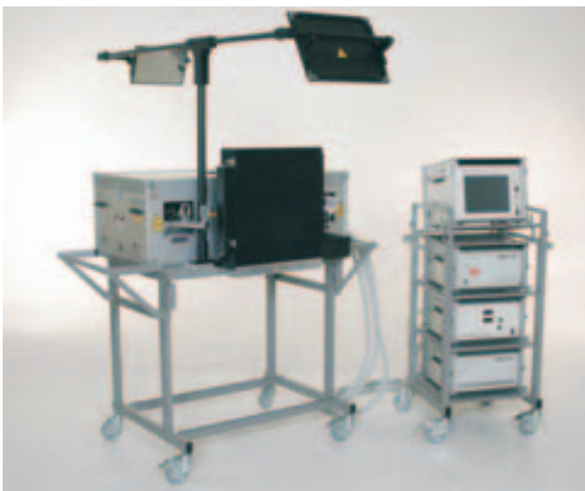
Fig. 1: Mobile holographic camera HSF-mini developed in cooperation with GEOLA, Lithuania.
