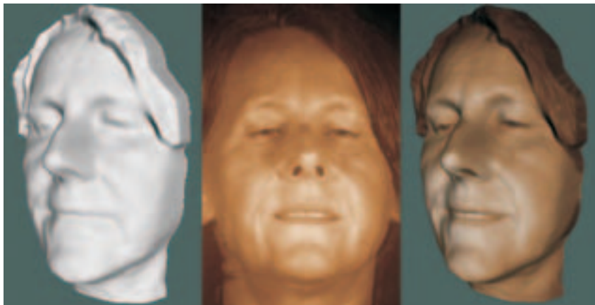
Fig. 6: The textured 3d model is a combination of the surface with the inherent greyscale texture of the hologram.
