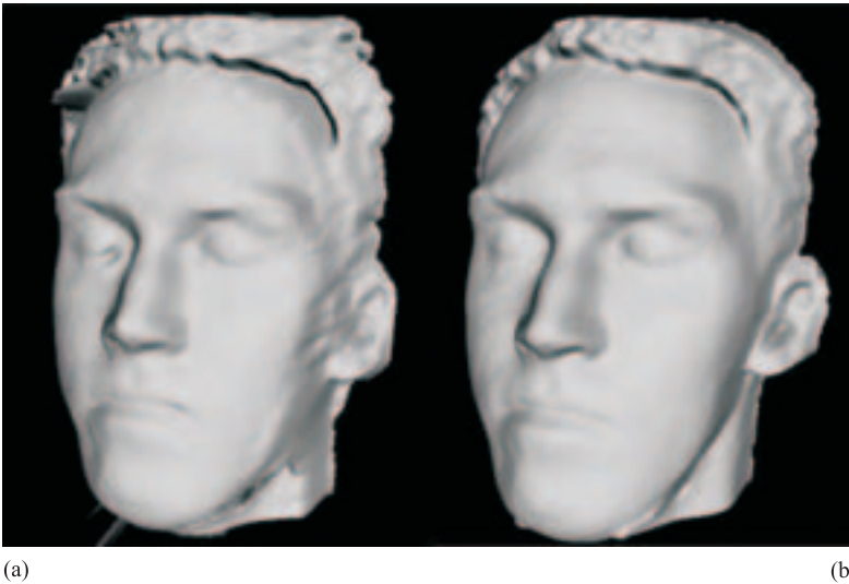
Fig. 7: Computer models obtained in a maximisation procedure parallel to the optical axis (a) and for each point along the iteratively calculated direction of image formation (b).
